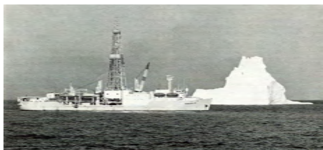
SEDCO/BP 471, was completed for commercial ocean drilling in 1978. The ship, 143.3 meters long, 21.3 meters wide, and with a draft of 7.3 meters and a displacement of 16,906 tonnes, was later converted for use by the Joint Oceanographic Institutions for Deep Earth Sampling (JOIDES) and renamed Resolution. This photograph was taken in Baffin Bay during Leg 105 of the Ocean Drilling Program.
